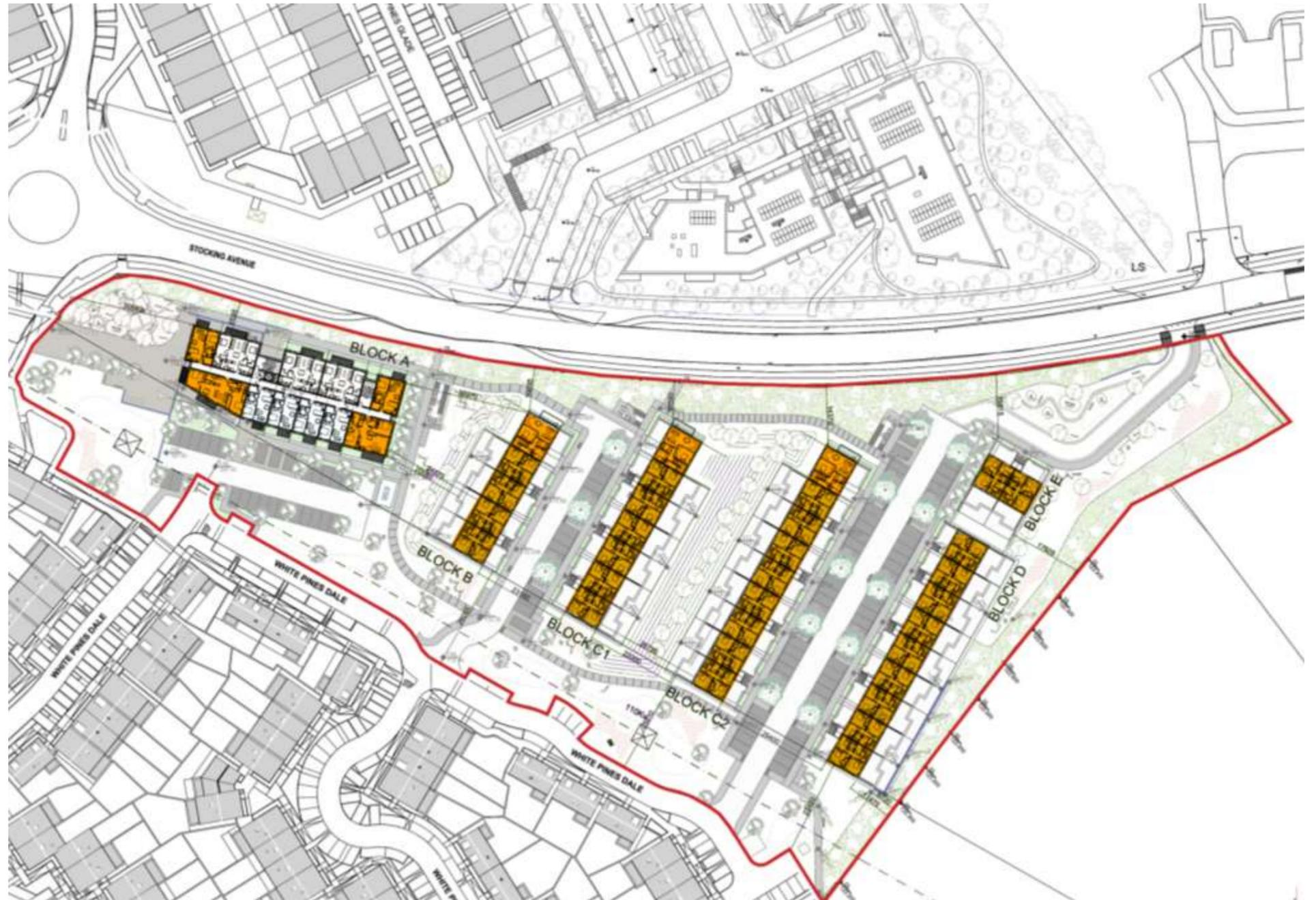
Figure 7 - First Floor layout showing dual aspect units
